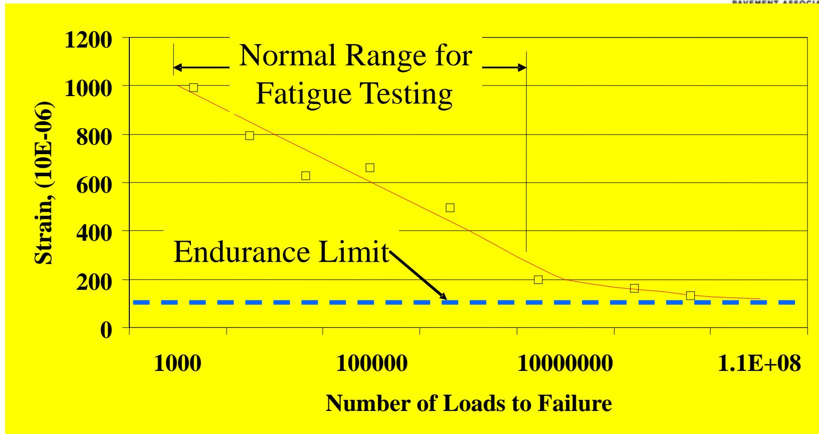
Normal Fatigue Testing Results Versus
